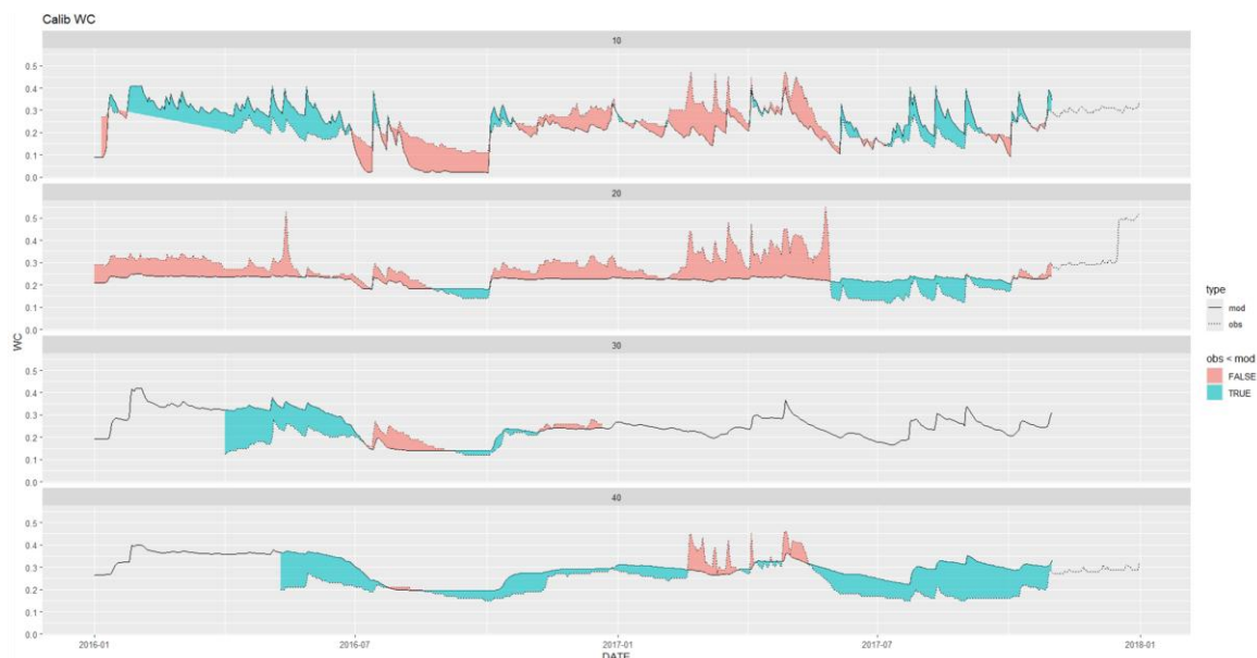
Figure 7.2. Modelled vs. observed soil water contents in the 10, 20, 30 and 40 cm layers at the Cechtnicky experimental site. Red and light blue colours indicate under- and overestimation, respectively.
