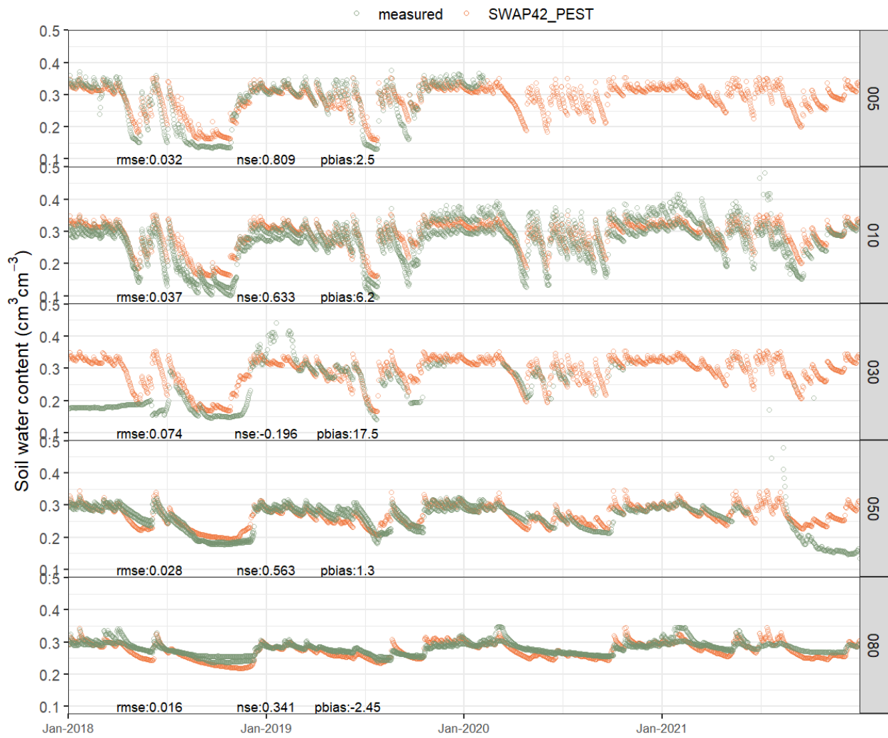
Figure 8. Validation of soil hydraulic parameters using PEST at the depths of 5, 10, 30, 50, and 80 cm. Crop: grassland.
